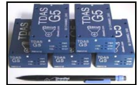
WorldSID Data Acquisition System, 160 data channels
