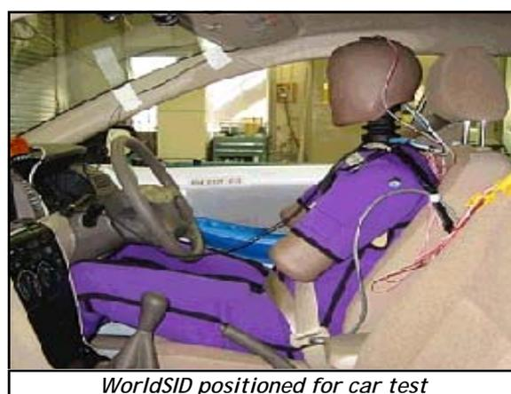
*WorldSID positioned for car test*
