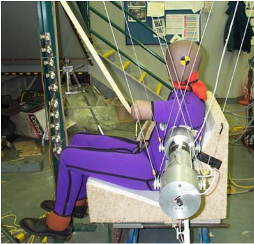
ISO TR9790 pendulum test on WorldSID
