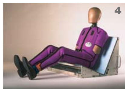
1. WorldSID during a full scale car air bag test. 2. WorldSID side impact biofidelity sled test. 3. WorldSID without a suit. 4. WorldSID with test suit. 5. Overlay of the WorldSID geometry and the UMTRI model.
